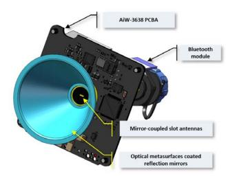
The performance of this antenna is sufficient for the measurement of liquid/solid levels in the range of 20M.
