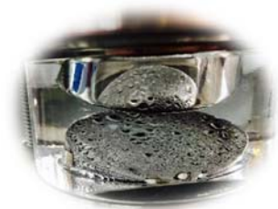
Water vapor condensation in the antenna
